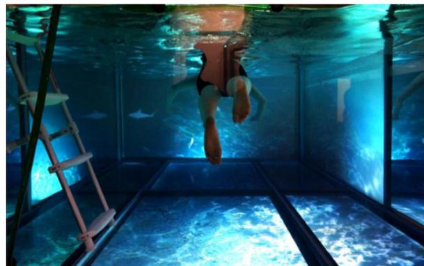
Figure 1. AquaCAVE: immersive environment for swimmers with multiple stereoscopic projections on surrounding acrylic walls
