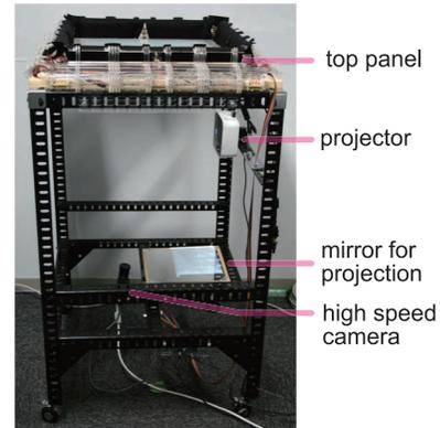
Figure 4: Z-touch hardware setup. The dimensions of Z-touch are  $1.0 \text{ m} \times 0.6 \text{ m} \times 0.6 \text{ m}$ . The framework is a 40 mm wide steel angle frame.
