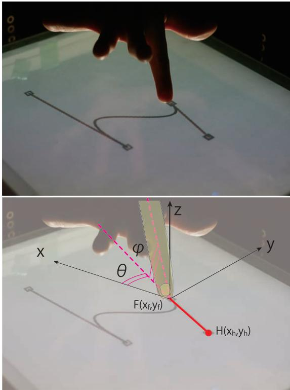
Figure 9: Bezier curve control. Endpoint of the curve is the contact position of the finger  $F(x_f, y_f)$ . The direction of the curve handle corresponds to the horizontal angle  $\theta$  of the finger. The length of the curve handle corresponds to the vertical angle  $\phi$ . Equation (2) relates the position of the endpoint  $F(x_f, y_f)$  and the position of the curve handle  $H(x_h, y_h)$ .
