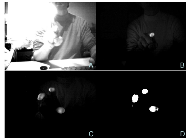
figure 5. Images taken by the "Light-Wall" configuration. (A: original image with an extremely shiny background, B,C: results of frame subtraction, D: after binarization)
